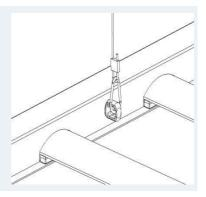
Use two people to lift the LED fixture to snap together or wrap the hangers to the strong enough support structures. And hang the four lance hangers to get a balanced LED fixture.
